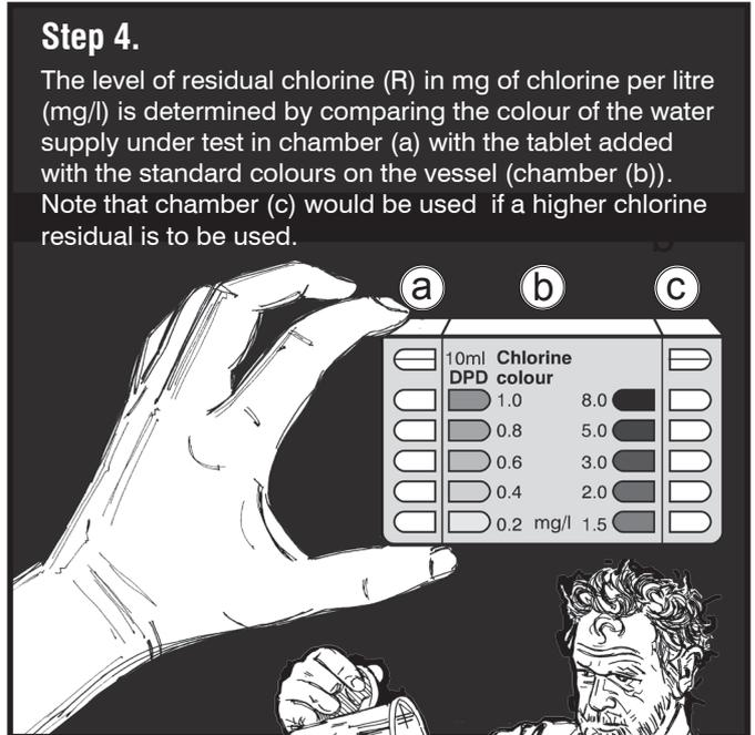
Figure 11.2. Steps in determining the chlorine residual in water using a comparator
