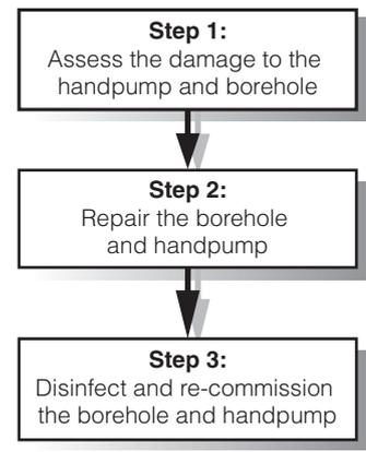
Figure 2.1. Steps for cleaning and disinfecting boreholes
