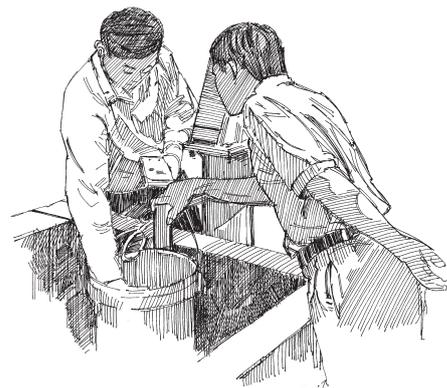
Figure 2.7. Checking the water for silt
