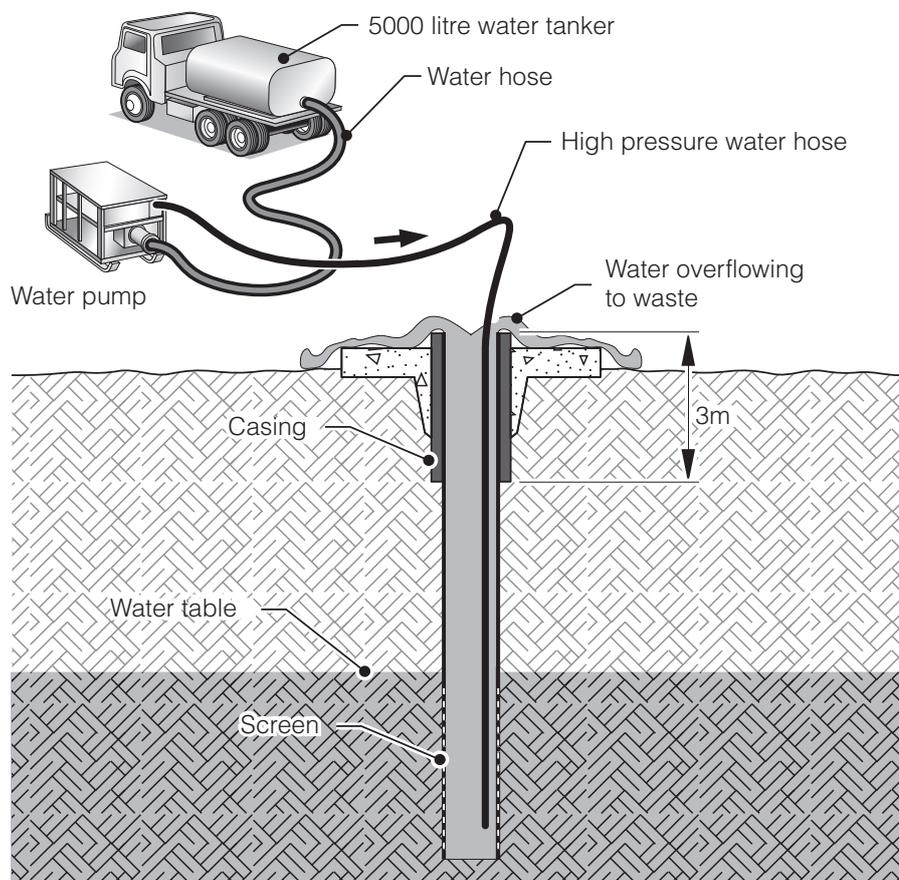
Figure 2.6. Flushing out a borehole by 'jetting'
