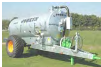
Figure 42. Trailer mounted storage tank
