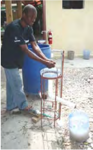
Figure 65. Oxfam prototype foot operated hand washing device with drain and container for waste water
