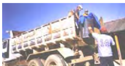
Figure 50. Dedicated emptying vehicle for urine diverted waste
