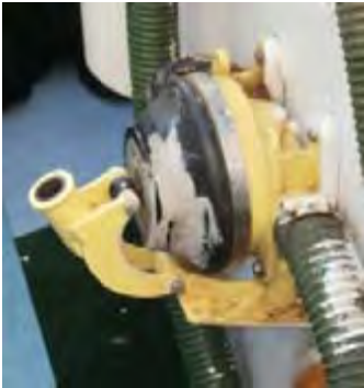
Figure 44. Typical manual diaphragm pump
