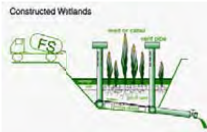
Figure 60. Cross section through a constructed wetland
