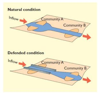
Figure 2.3 Flood defences should not be considered in isolation. Source: Fleming (2002b, p18)
