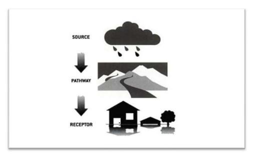
Figure 2.1 Source-pathway-receptor model for floods: the greatest control is with the receptor. Source: Huntingdon and MacDougall (2002)
