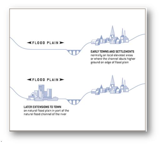
Figure 2.5 Riverside settlements encroaching on the flood plain. Source: Fleming (2002b, p16)
