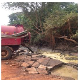
Figure 20: Vacuum truck discharging into the environment next to STP
