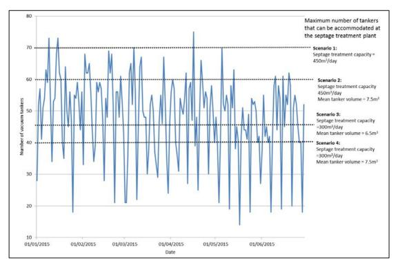
Figure 16: Number of tankers discharging to Dompease STP over six months in 2015, compared with the number of tankers that can be accommodated under 4 different scenarios (Furlong, 2015a).
