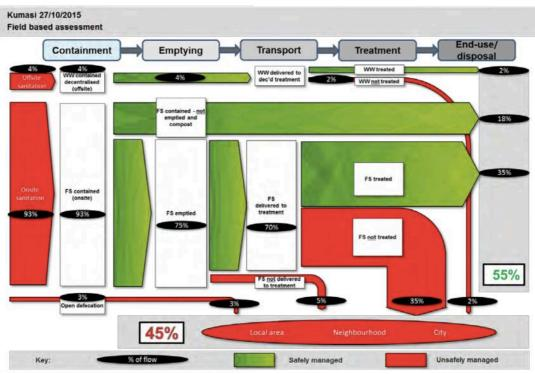
Figure 1: SFD Example. SFD of Kumasi, Ghana (Furlong, 2015a)
