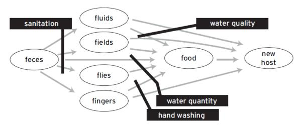
Figure 2.5 The F-Diagram: Transmission Routes for Infection
