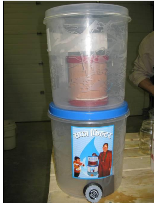
Filter with one ceramic candle
