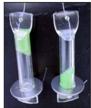
Box Cooker and Water Pasteurization Indicator (WAPI) (Credit: Solar Cooker International)
