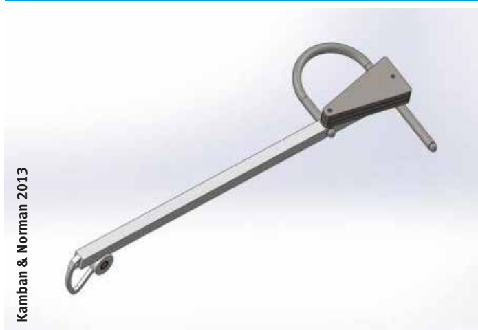
Figure 13: Design of adapted 'p' pump handle. User sits on 'U shape' side
