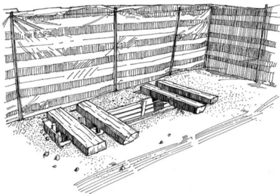
**Figure 3.** A simple trench latrine: an immediate action to an urgent situation
