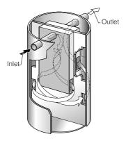
Figure 11. Examples of pre-fabricated septic tanks
