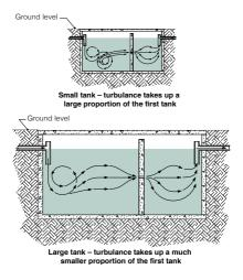
Figure 6. A comparison of the effects of turbulence on small and large tanks
