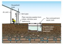
Figure 1. Wastewater treatment using a septic tank
