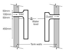
Figure 8. Tank inlet and outlet pipes
