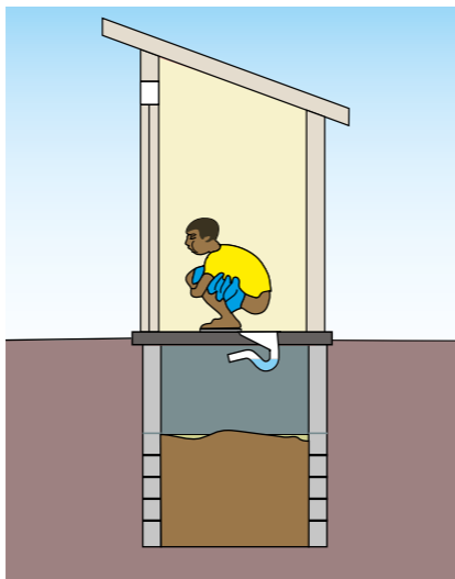
Figure 3. A direct pour-flush latrine
