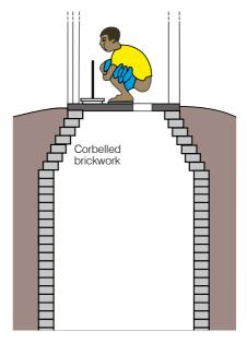
Figure 5. Pit with corbelled lining
