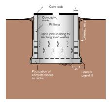
**Figure 2.** Details of the construction of a shallow pit with lining
