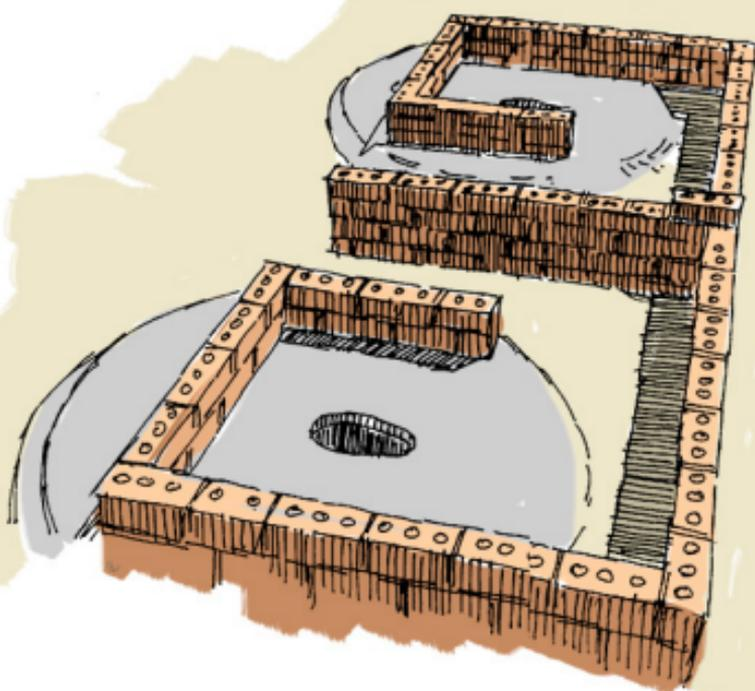
Ideally, the superstructure or shelter should be placed so that it does not rest on the slab, as this will add extra load. The slab will have to be stronger if it does have to support the superstructure. It would also mean that the whole structure would have to be demolished to gain entry into the vault.
