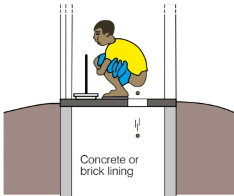
**Figure 3.** Well-supported slabs can be smaller
