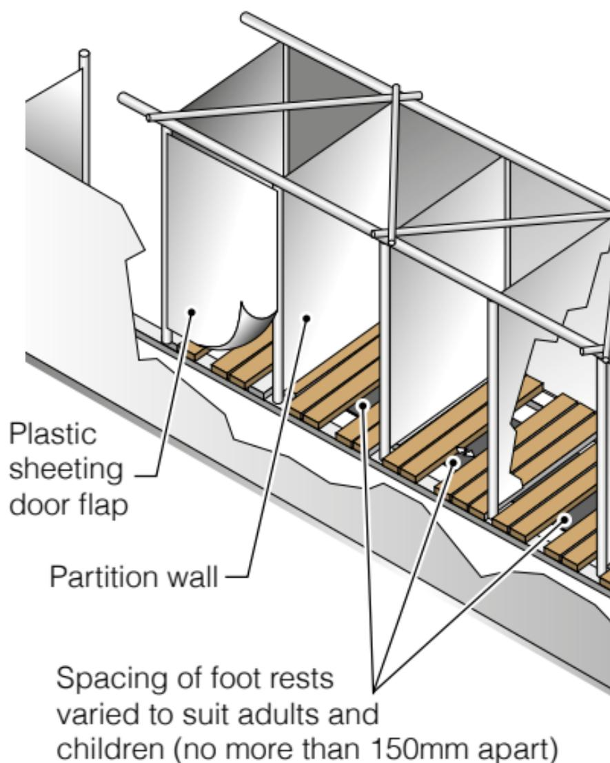
**Figure 6.** Temporary wooden slabs may only be acceptable in the initial stages of an emergency
