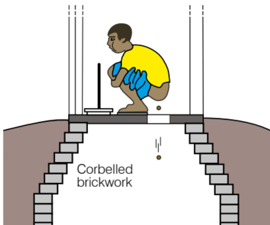
**Figure 4.** Corbelled brickwork lining
