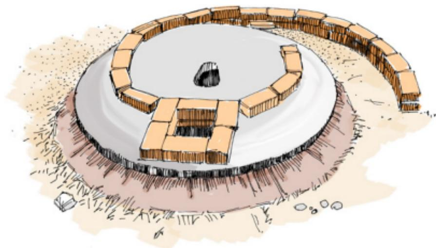
**Figure 1.** A round slab providing the foundation for part of the wall of the superstructure
