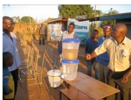
Figure 4. Table top water filter as produced in Ethiopia, Malawi and Kenya
