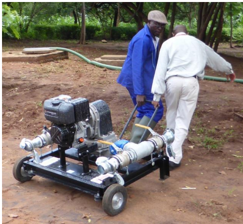
Photograph 3. Diaphragm sludge pump
