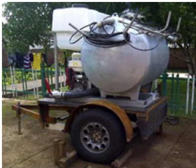
Photograph 1. ROM vacuum machine
