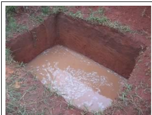
Photograph 3. When it rains the pit fills up and water is infiltrating in the ground
