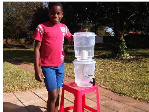
Photograph 6. Self-supply water can be made safe to drink with low cost filters like this Filter produced in Malawi
