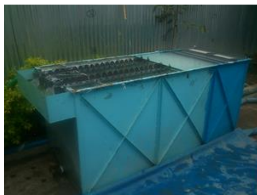
Photograph 2. Modified IPS prototype with hydraulic flocculator extension and overflow launders
