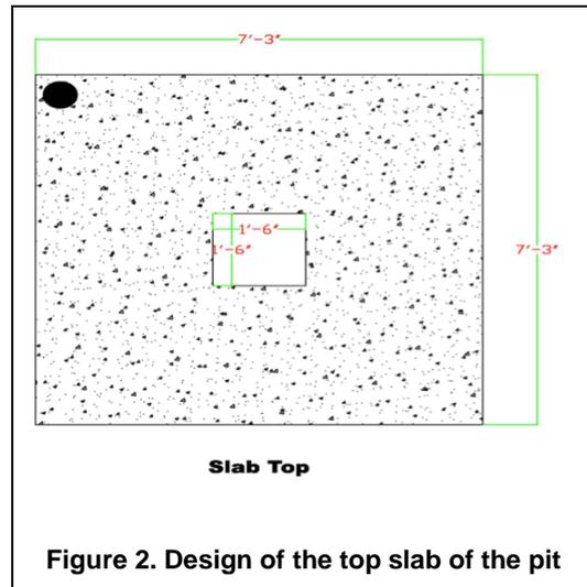
Figure 2. Design of the top slab of the pit
