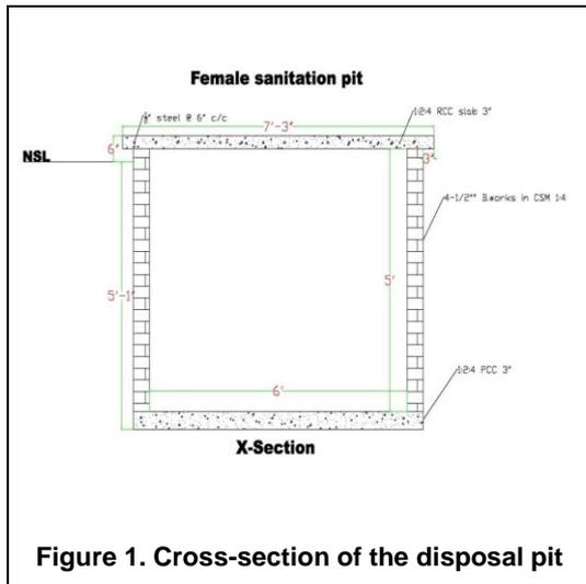
Figure 1. Cross-section of the disposal pit
