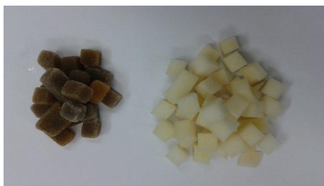
Photograph 1. DHY-1 carrier material (left: carrier materials with microorganism; right: carrier materials without microorganism)
