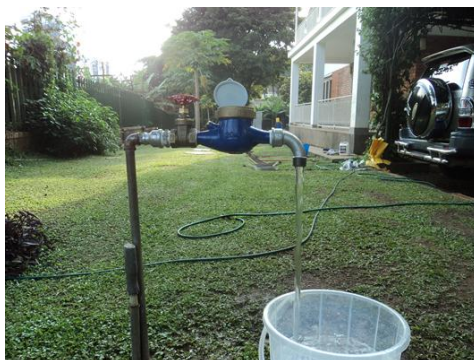
Photograph 1. Calibration of water meter using a 20-litre graduated bucket; water meter connected to a tap
