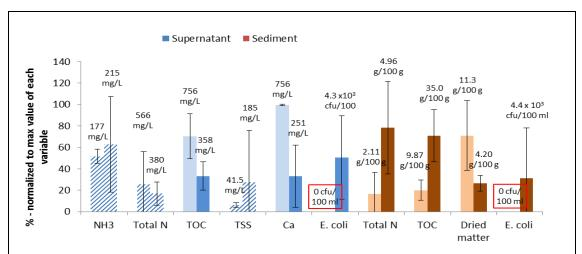
Figure 6. Characteristics of supernatant and sediment after incubation. For each parameter, the left column is average of high lime-amended ("high treatment", 0.5 and 1.5 % w/v lime) incubations and the right column is average of control and amendment at 0.1 % (w/v) lime ("low treatment"). Hashed columns are not significantly difference. Solid fill represents difference at p(same) < 0.05.
