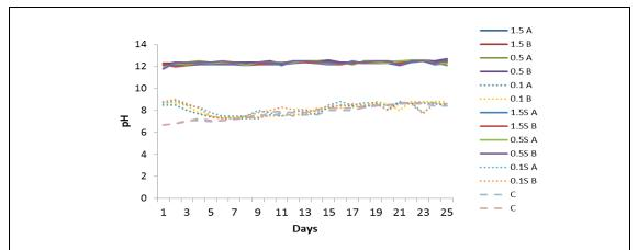
Figure 5. Effect of initial lime concentrations on pH over a 25 day incubation. A, B: duplicate incubations at the same concentration. S: lime added as a slurry C: unamended control.
