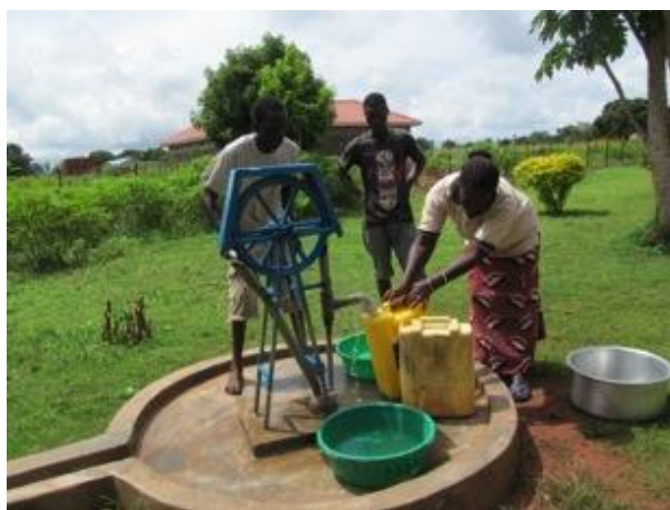
Photograph 3. The new family rope pump model at Watmon's home. His wife, Peri is selling the water to customers
