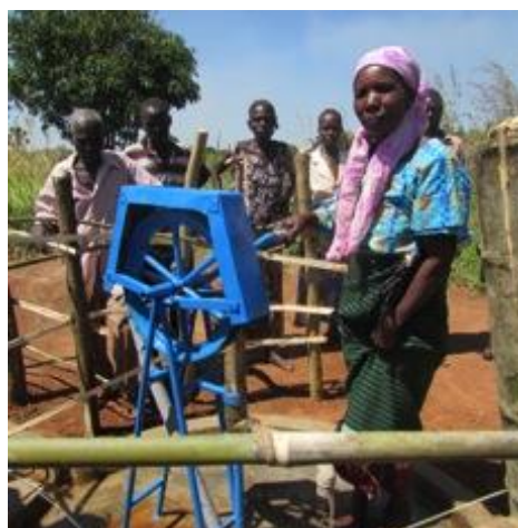
Photograph 4. The new communal rope pump model at Abili East Village
