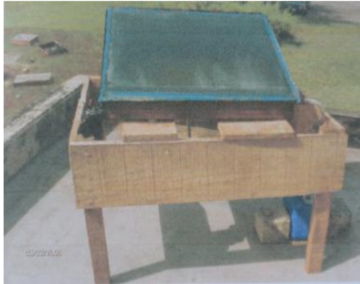
Photograph 1. Constructed solar still
