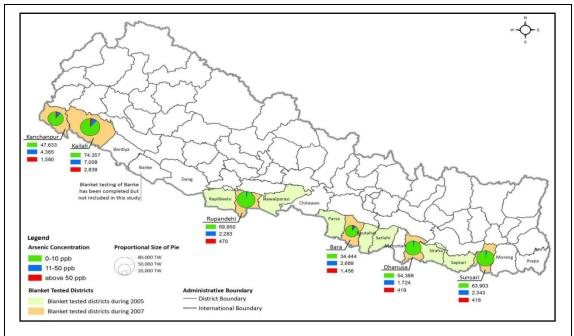
Figure 1. Arsenic contaminations in tube wells of six districts of Terai region of Nepal
