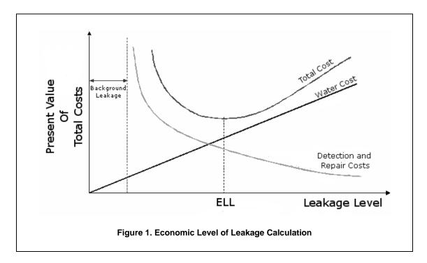
The ELL may be calculated on the basis of the financial costs to the utility, which demonstrates the value to the utility of reducing the leakage of water that has been treated and pumped incurring the cost of energy and chemical bills etc. Alternatively ELL may be calculated on the basis of economic costs to society, which take account of the financial costs to the utility AND externalities like social and environmental impacts.
