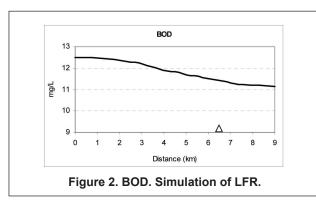
From Figures 1 and 2 it is seen that the influence of the discharge of treated wastewater is negligible in terms of BOD and DO, partially because the wastewater flow is small compared with the river flow, and partially because the effluent concentrations are low.
