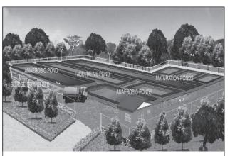
Figure 1. Septage treatment facility design using waste stabilization ponds for Dumaguete City, Philippines
