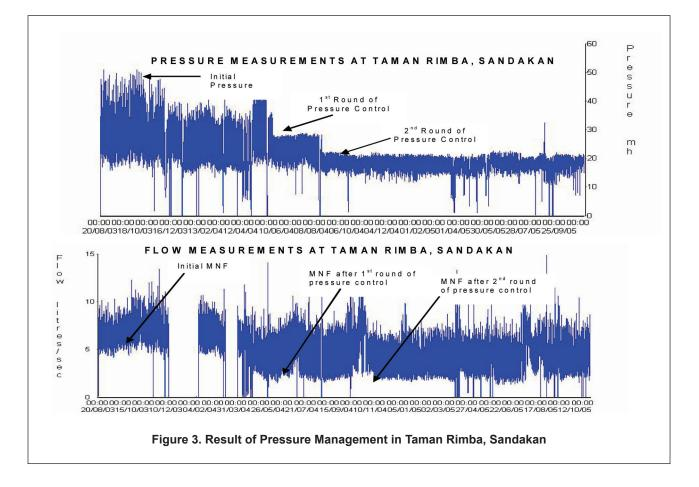
Sandakan is illustrated in Figure 3. MNF reduced as a result of pressure reduction.
