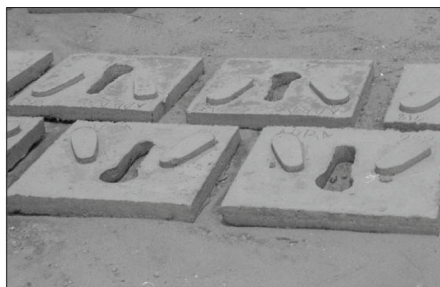
Photograph 2. San plat slabs
