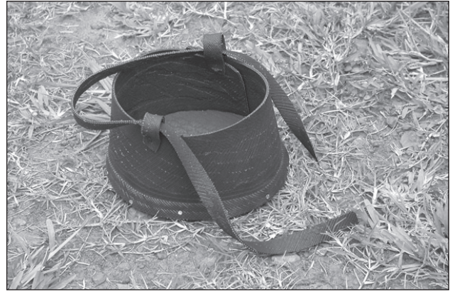
Figure 5. Knee cap made of recycled rubber tyres
