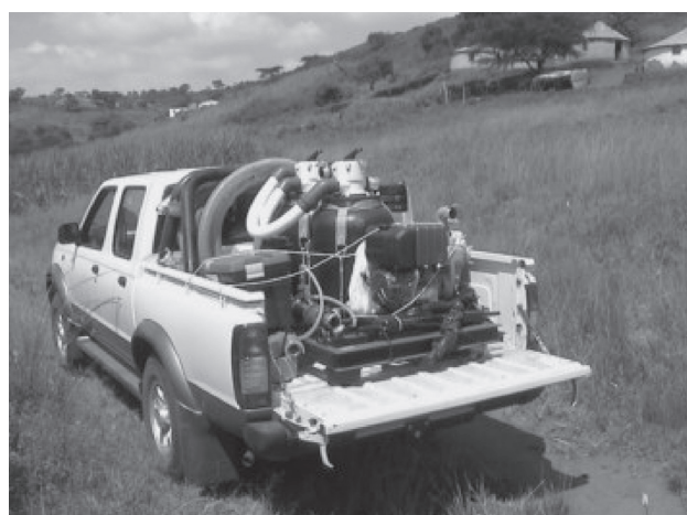
Fig. 2 Complete water treatment unit on pick-up car, Kwa Zulu Natal.
