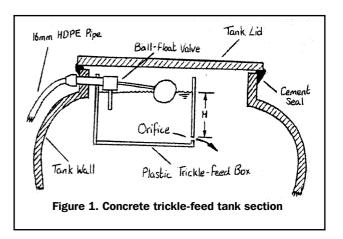
head of water ('H' on Figure 1) above the orifice, which causes a constant flow to 'trickle' into the tank.
