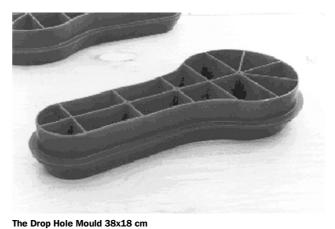
This mould is ideal for the round dome shaped SanPlats but can be used for any kind of SanPlats. As plastic moulds are identical all the lids will be well fitting, avoiding problems with smell and flies.
