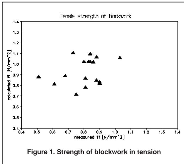
Figure 1. Strength of blockwork in tension
