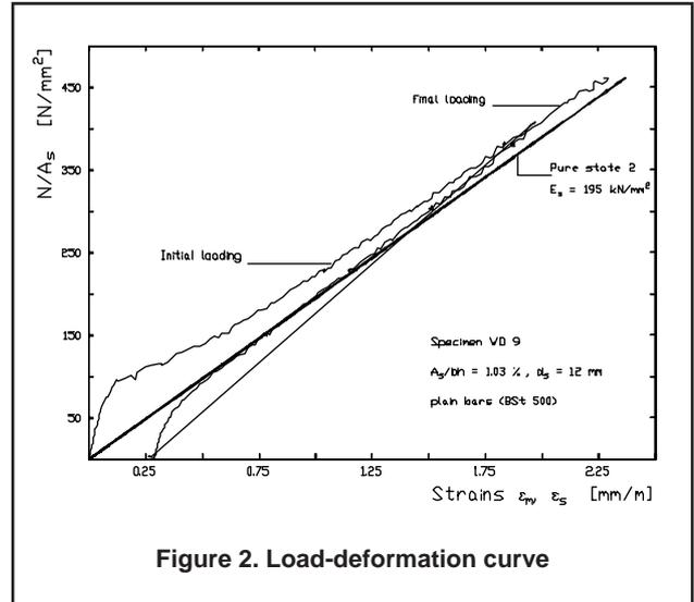
Figure 2. Load-deformation curve
