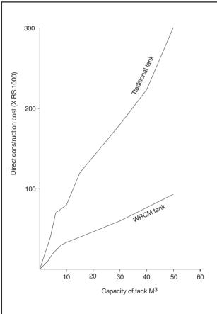
Figure 1. Capacity/cost of WRCM tanks compared to traditional tanks
