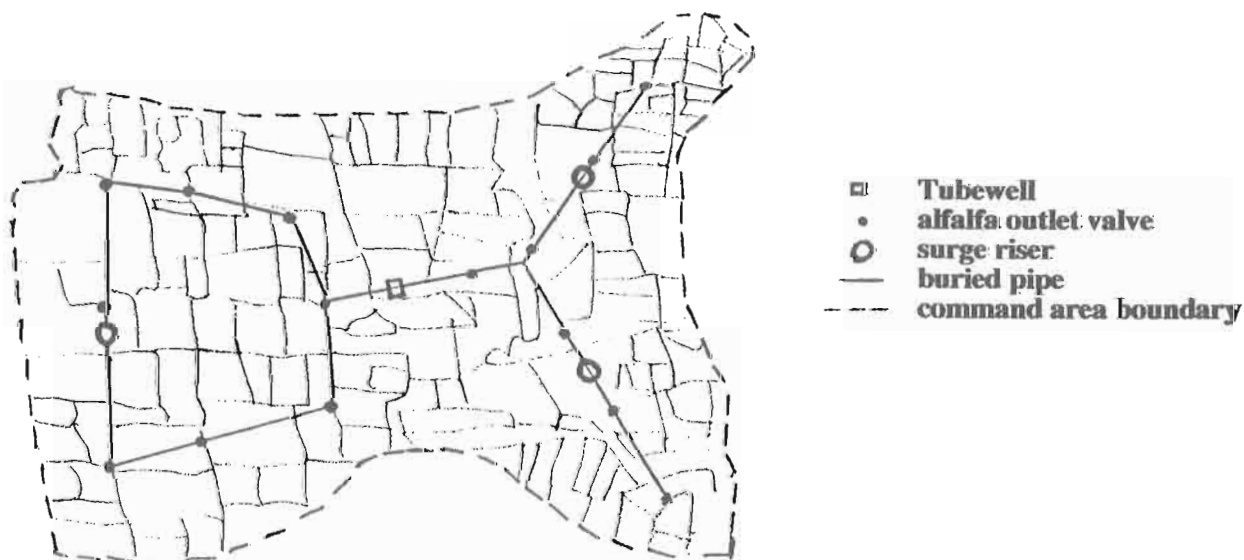
Figure 1. Buried pipe system layout with a loop system on the left side and a branching system on the right.
