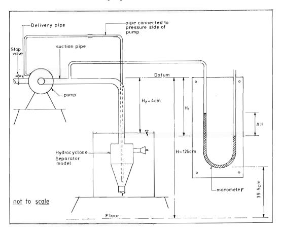
This arrangement influenced the removal efficiency of the cyclone. The water "pushed" back into the hydrocyclone tended to increase the downward axial velocity of the solid particles. The particle removal is independent of gravitational forces.
