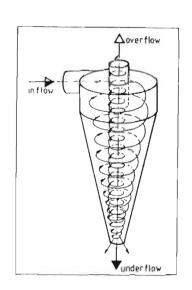
A modified hydrocyclone is introduced to remove the suspended solids often found in surface waters prior to reaching the pump or any other water raising machinery. The use of this hydrocyclone was tested in the hydraulics laboratories of the University of Dar es Salaam during the 1983/84 academic year. The results of the experiments show that this type of hydrocyclone can be used effectively in the removal of suspended solids.
