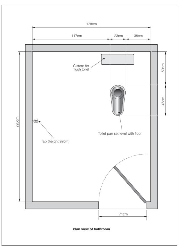
Figure 9.35. Dimensions of Mr Bakul's bathroom/toilet.
