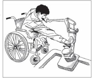
Figure 6.1. Handpump sited close to edge of apron.
