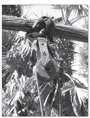
Figure 6.8. Detail of pulley lifting mechanism. (Case-study 9.12, page 191)
