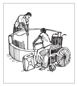
Figure 6.11. Well wall of different heights.
