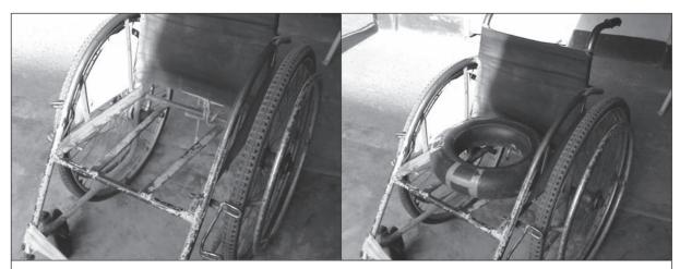
Figures 6.66 and 6.67. Wheelchair convertible to a bathing seat. Wheelchair with cushion and seat board removed and tyre inner tube in place. *(Case-study 9.3, page 164)*
