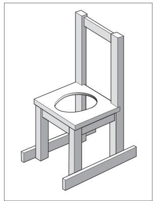
Figure 7.37. Toilet chair with side runners. These spread the weight of the chair and improve stability.
