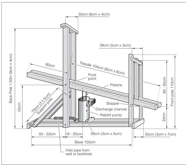
Figure 9.60. Treadle pump.
