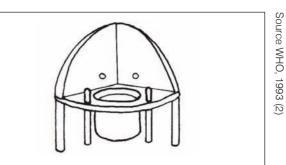
Figure 7.50. Corner seat with potty insert for child with poor sitting balance.
