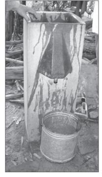
Figure 9.59. Sand water filter.
