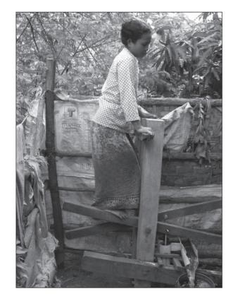
Figure 6.10. Treadle pump in operation. (Case-study 9.13, page 193)
