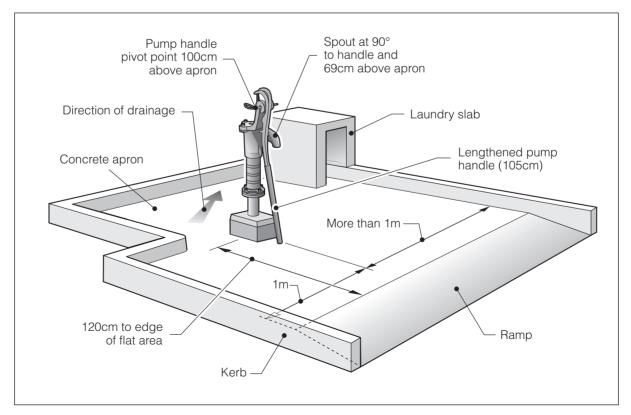
Figure 9.21. Layout of CRP handpump apron.
