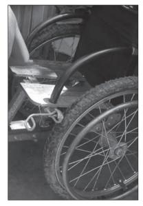
Figure 9.75. Wheelchair seat with central plank removed.
