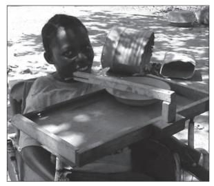
Figure 6.75. Implement holder attached to wheelchair tray, used with spoon, toothbrush or other tool. (Case-study 9.27, page 237)
