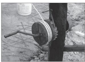
Figure 6.9. Detail of ratchet and pawl winding mechanism. (*Case-study 9.11, page 187*)
