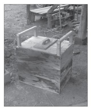
Figure 7.15. Wooden toilet seat with handrails. *(Case-study 9.17, page 209)*
