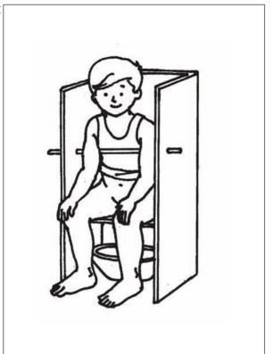
Figure 7.22. Toilet chair with removable horizontal bar to prevent user falling forwards.
