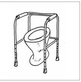
Figure 7.13. Four legged tubular steel frame, with cushioned handles and rubber 'feet'. Adjustable height.
