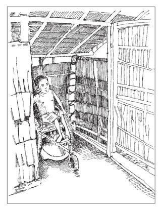
Figure 5.26. Toilet with space to position wheelchair over toilet, but not beside it. The user must reverse in. (Case-study 9.15, page 201)
