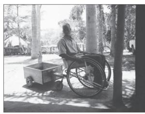
Figure 6.29. Two-wheeled wooden wheelchair trailer.
