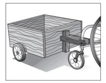
Figure 9.151. Detail of trailer hitching arrangement.
