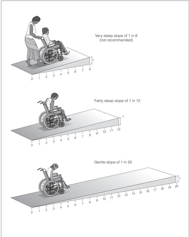
Figure 5.3. Slope gradients.
