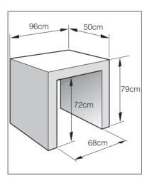
Figure 9.17. Dimensions of laundry slab.
