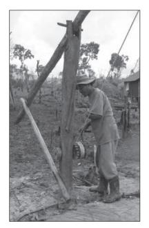
Figure 9.48. Mr Ath turns handle of winding mechanism to lower and lift bucket.
