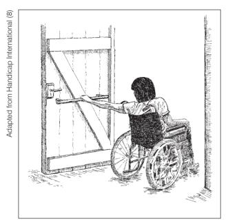
Figure 5.21. Door-rail extending the full width of the door.
