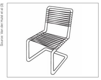
Figure 6.54. Steel tube frame bathing chair with seat and back of woven plastic strips.
