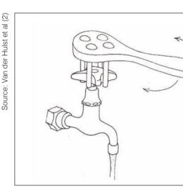
Figure 6.21. Tap turner made by driving nails through a piece of wood.
