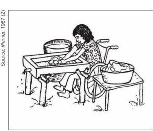
Figure 6.84. Concrete or wooden washstand with ridged bottom for washing clothes.
