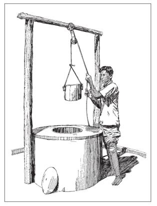
Figure 6.7. Rope and pulley over a shallow well. (Case-study 9.12, page 191)
