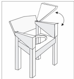
Figure 7.20. Chair with hinged side-rails that can be raised out of the way.
