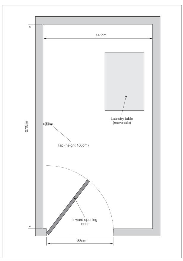
Figure 9.25. Layout of laundry/bathroom.
