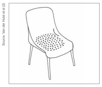
Figure 6.53. Moulded plastic bathing chair with holes in seat.
