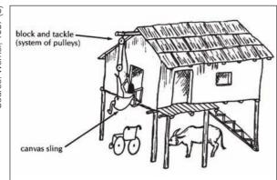
Figure 6.31. Rope and pulley system could be used to lift water, or even people.
