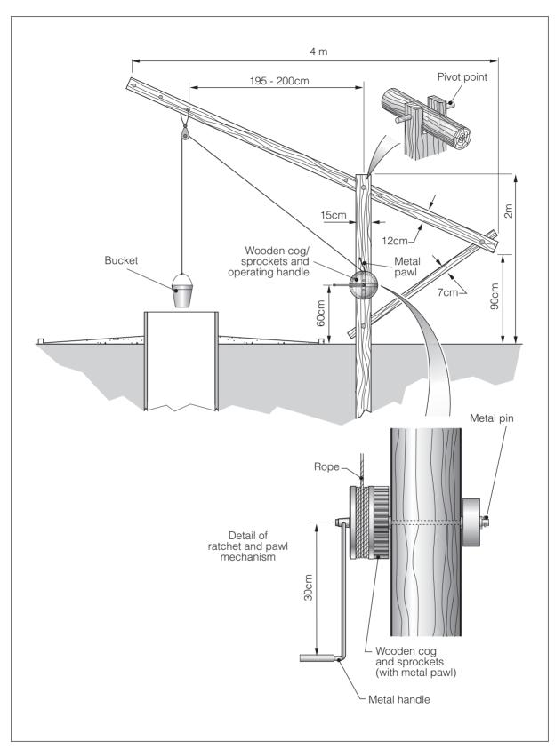
Figure 9.51. Well with ratchet and pawl lifting mechanism.
