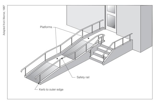
Figure 5.4. Ramp with mid-level resting platform.
