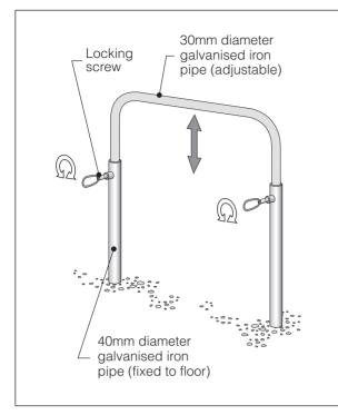
Figure 7.18. Detail of adjustable joint.
