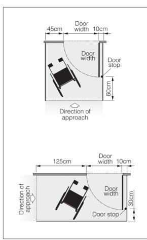
Figure 5.15. Minimum dimensions of flat platform for opening a door.
