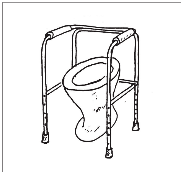
Figure 7.13. Four legged tubular steel frame, with cushioned handles and rubber 'feet'. Adjustable height.
