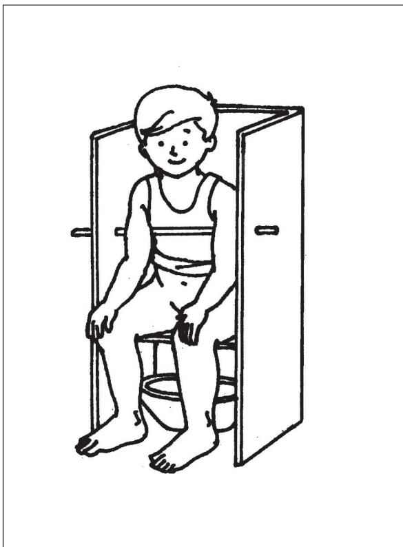
Figure 7.22. Toilet chair with removable horizontal bar to prevent user falling forwards.
