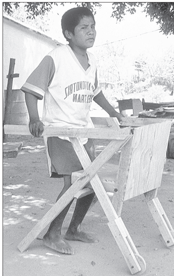
Figure 7.51. This child uses walking frame that converts to a toilet seat (below). The fold-down seat has a potty insert which he can use, wherever he is at the time.
