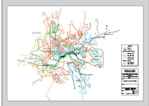
The map indicates 6 supply zones that are demarcated by blue, red, green, yellow and purple lines. Each of these lines is drawn to indicate supply zones that are isolated from one another by cut off valves.
