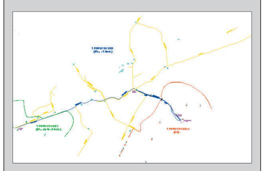
The system comprises of primary and secondary distribution mains (marked as blue and yellow on the map). The primary transmission main begins at the water treatment works and feeds two service reservoirs and one supply tank. The principal secondary mains are marked as yellow. The green and red lines demark supply zones within the network.
