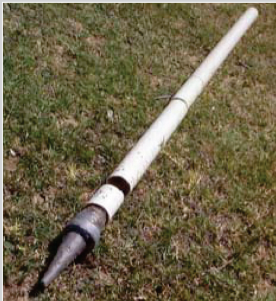
Photograph 5.2. Well-point fracture between transverse slots
