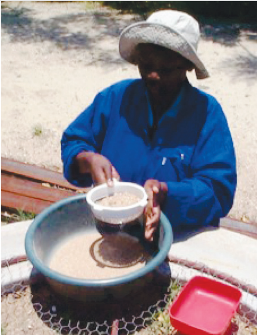
Photograph 3.8. Simple grading test using household sieve
