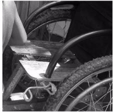
Figure 19. Heng's wheelchair with removable centre panel in seat to create a toilet seat.
