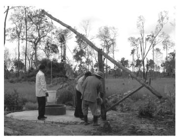
Figure 4. Mr Ath Vuth demonstrates the fixed cantilever well that he designed and constructed himself.
