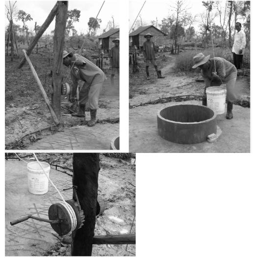
Figure 5. Ratchet and pawl mechanism, constructed out of wood by Mr Ath.
