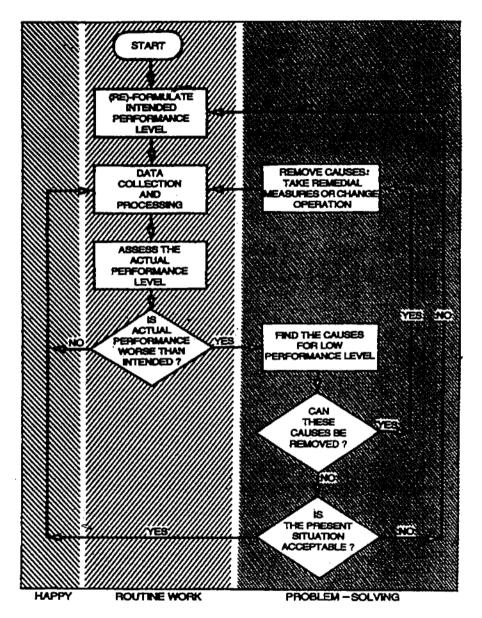
Figure 1.4. A simple flow chart of irrigation water management
