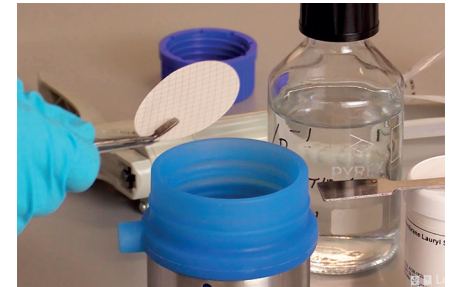
Figure 13. Placing the filter into the unit
