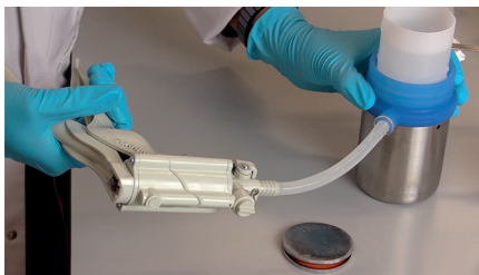
Figure 17. Operating the vacuum pump
