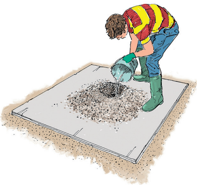
Step 10. Pouring more water into the crater
