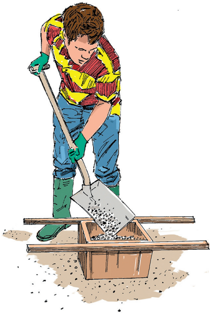
Step 2. Filling the container with aggregate
