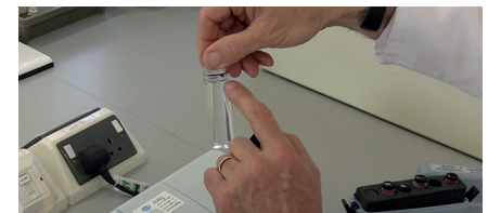
Figure 27. Face the black triangle towards you
