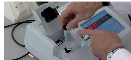
Figure 23. Placing the tube into the turbidity meter
