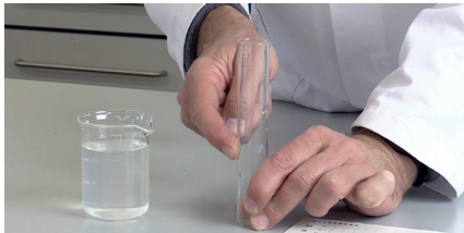
Figure 10. The Chinese turbidity tube
