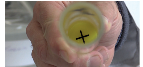
Figure 6. A black cross marked at the base of the inside of the tube
