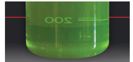
Figure 1. A jar containing fluorescein: light passing through is not scattered
