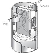
**Figure 11.** Examples of pre-fabricated septic tanks
