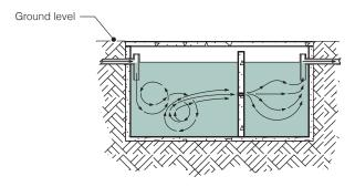
Small tank - turbulance takes up a large proportion of the first tank
