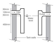
Figure 8. Tank inlet and outlet pipes
