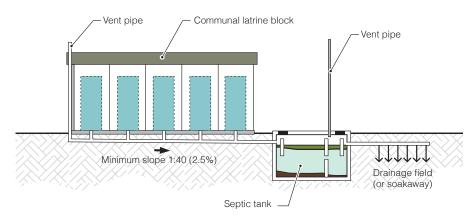
Figure 2. Communal toilet connected to a septic tank and drainage field
