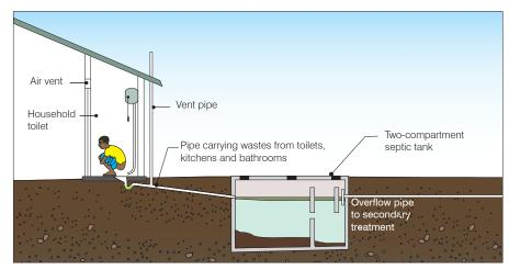
Figure 1. Wastewater treatment using a septic tank
