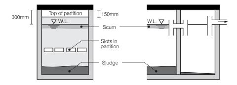
Figure 10. Options for flow through tank partitions
