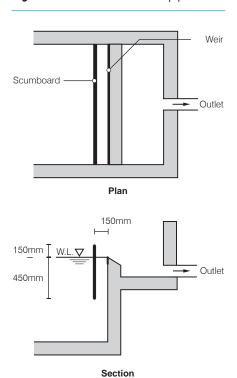
Figure 9. Tank outlet using overflow weir
