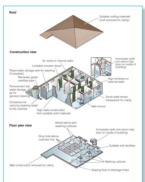
**Figure 3.** Schematic views of a sanitation block for girls including cubicles for bathing and washing
